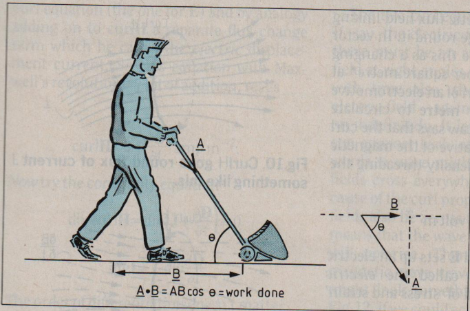
Fig.6. Work done by the component of a force shows a typical example of the scalar product of two vectors.
