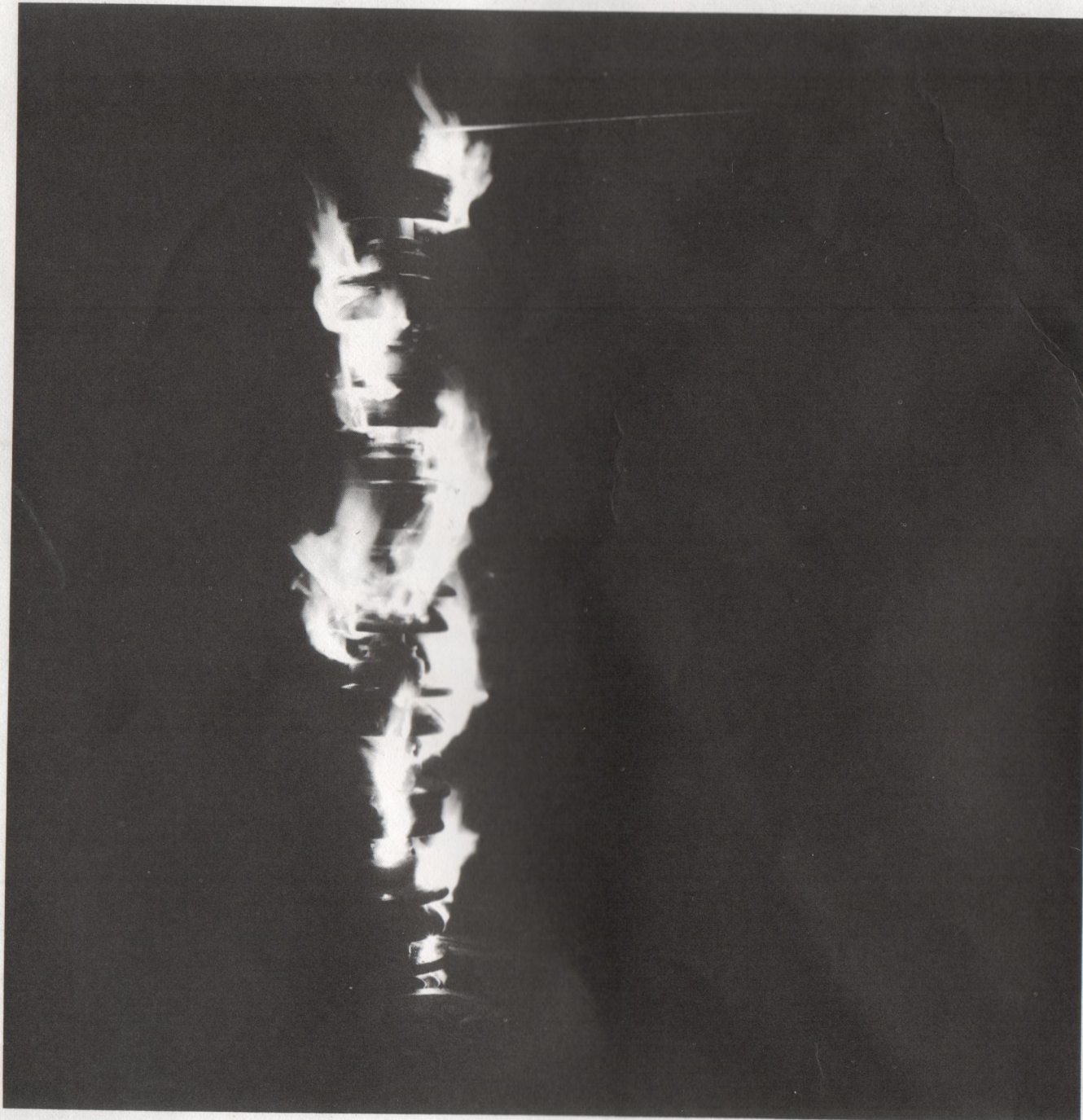
Arcing across a wet high-voltage insulator under test (left)
